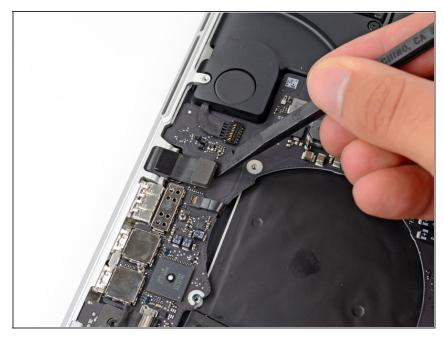
Use the flat end of a spudger to pry the headphone jack connector up from its socket on the logic board.
